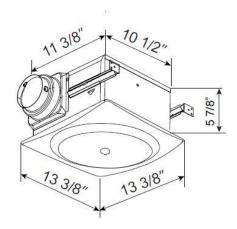
ETL Listed for installation over tub/shower enclosure with GFCI circuit wiring.
